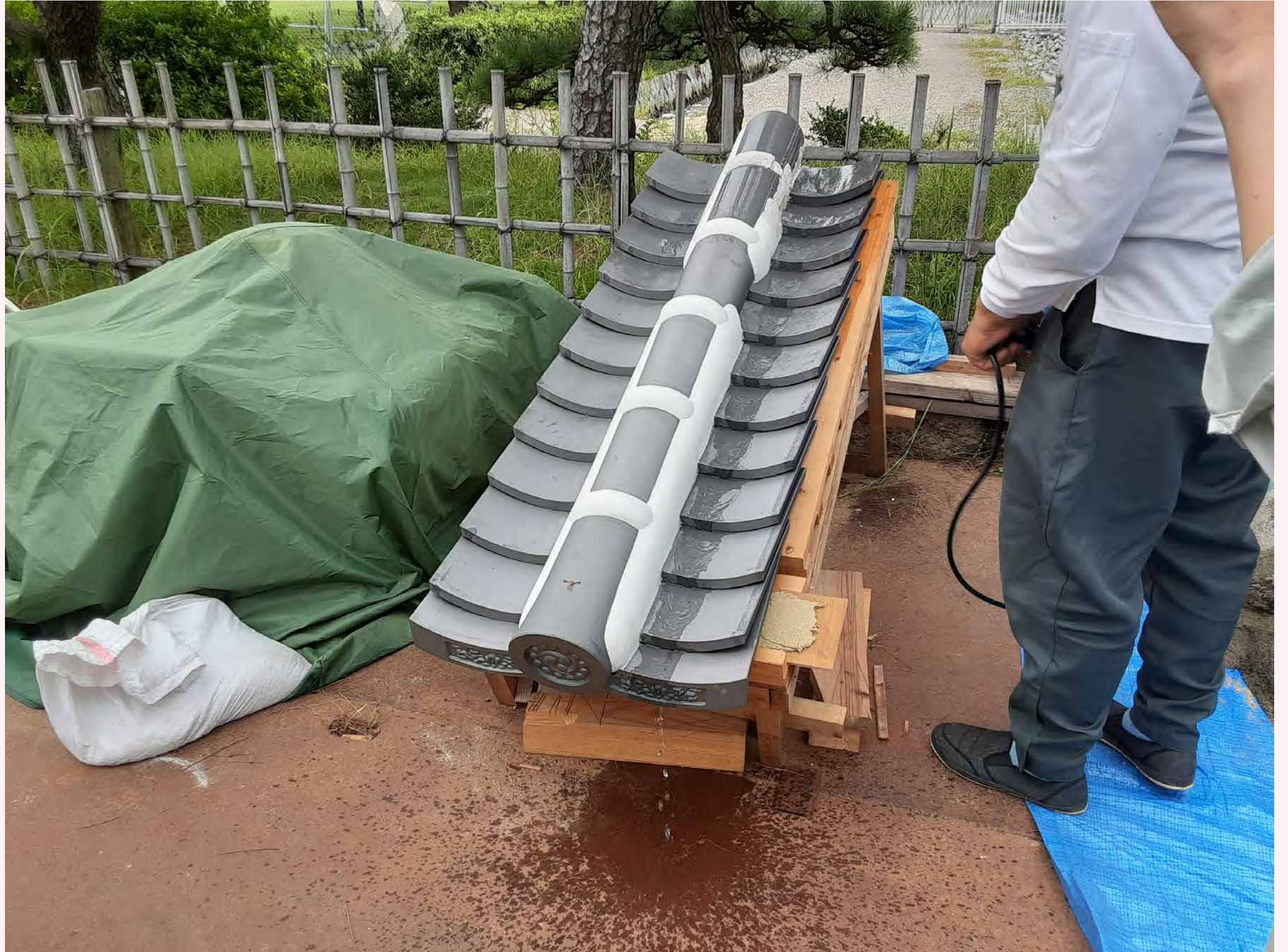
Rainwater Drainage Test Using Model
