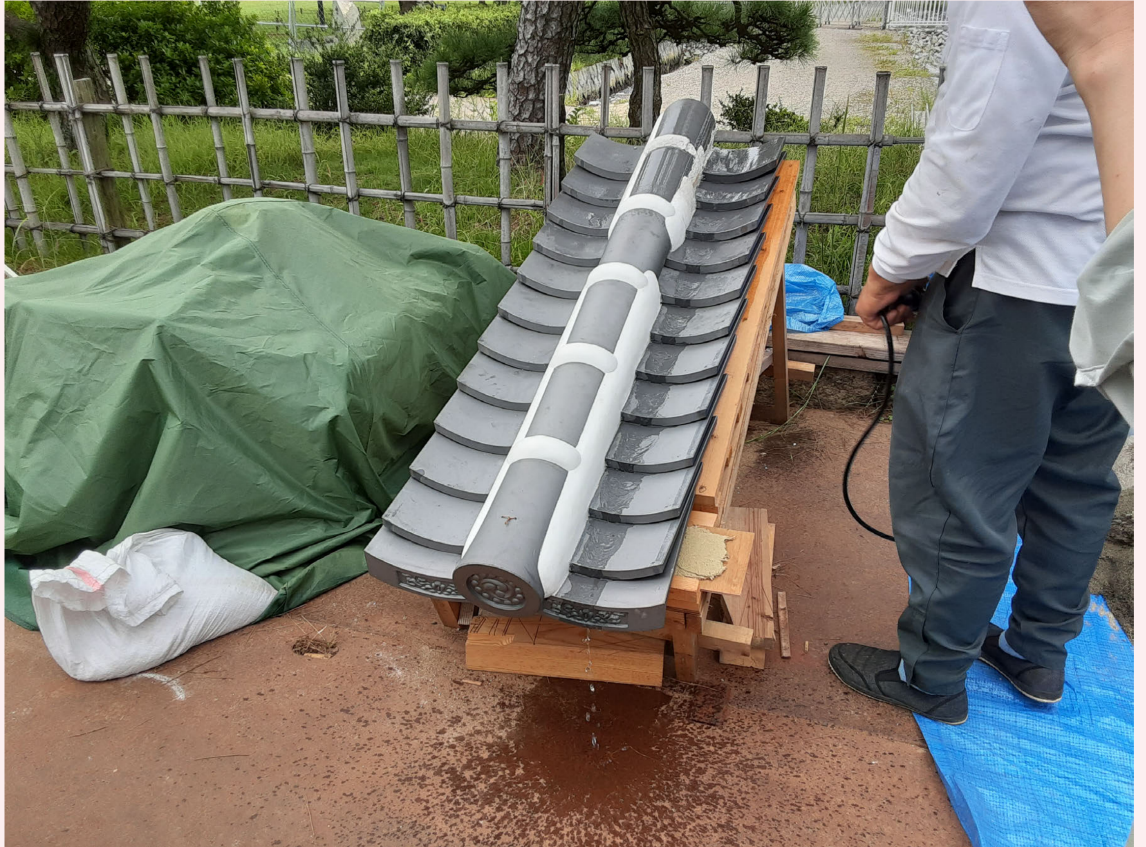
Rainwater Drainage Test Using Model
